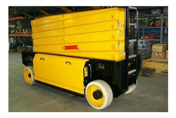
It is mandatory to use the support during work carried out close to the scissors, if the platform is in an elevated state.
