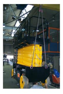
The crane eyes should be used as rope fixing points after loading it onto a transport vehicle.
