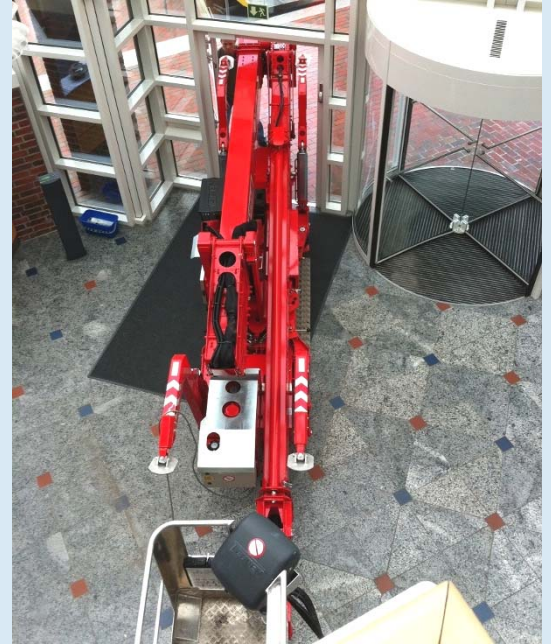
With its compact dimensions the LEO23GT fits through most entrance doors. The sensitive electro-proportional controls allow precise maneuvering.
