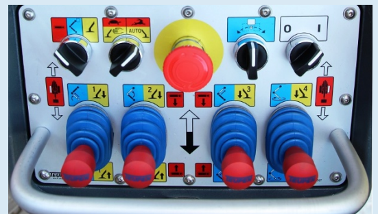
A clearly arranged control panel with color coded functions and only four joysticks for the entire lift operation supports intuitive and safe handling even for inexperienced users.
