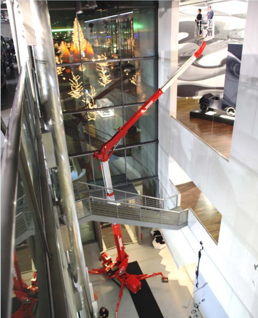
The light LEO23GT can be towed on standard trailers. It can either be driven on the trailer or simply use its outrigger system.
