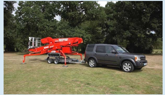
The light LEO23GT can be towed on standard trailers. It can either be driven on the trailer or simply use its outrigger system.
