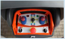
Teupen controls are well-arranged with color coded functions. Only two joysticks and one switch for the entire lift operation.
