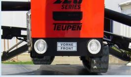
The adjustable track chassis allows driving safely alongside slopes and to increase ground clearance for better terrainability.
